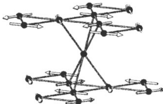
Figure 59 The magnetic structure of Gd_2Ti_2O_7 at 50 mK showing the Kagome type planes separated by paramagnetic Gd^{3+} ions on a planar triangular lattice. (Reprinted with permission from J.M.D. Champion, A.S. Wills, T. Fennell, S.T. Bramwell, J.S. Gardner, M.A. Green, Phys.Rev. , 2001, B64 , R140407. © 2001 by the American Physical Society)
