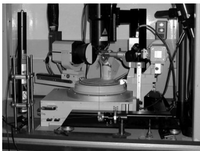
Figure 14 An experimental setting for single-crystal X-ray diffraction study at 30 K, showing a Bruker three-circle diffractometer with a SMART 1000 CCD area detector, a laser device for crystal irradiation and a HeliX open flow helium cryostat in action
