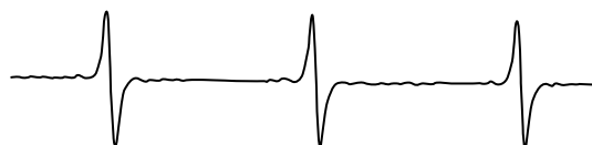
Figure 3 Solution spectrum of a typical nitroxide radical where the unpaired electron is mainly interacting (i.e., hyperfine interaction) with the nitrogen nucleus. Since nitrogen is predominantly the 14 N isotope, the line is equally split (hyperfine splitting constant) into three ( m_I = +1, 0, -1 ) lines
