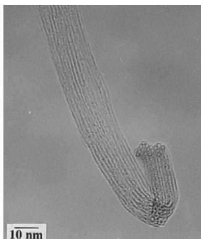
Figure 8 TEM of SWNTs bundle synthesized using Ni:Y (2:0.5 at.%) catalyst. (Reprinted from Ref. 47. © 1998, with permission from Elsevier)
